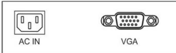
VGA INPUT: D-SUB 15 pins Connector
