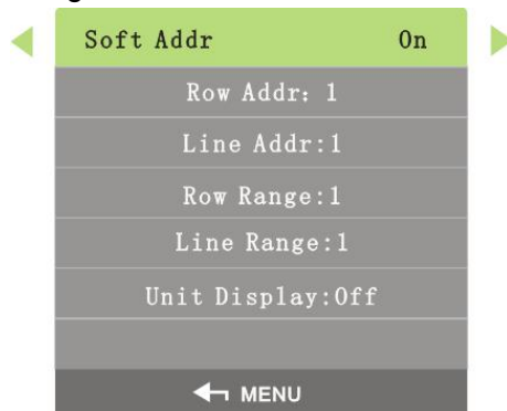
Figure 4-27 Soft address switch
