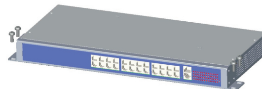
Figure 2-4 Fix the switch on wall
