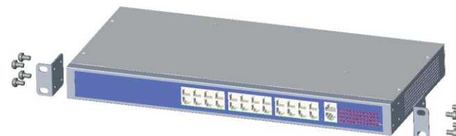
Figure 2-1 Install hangers diagram
